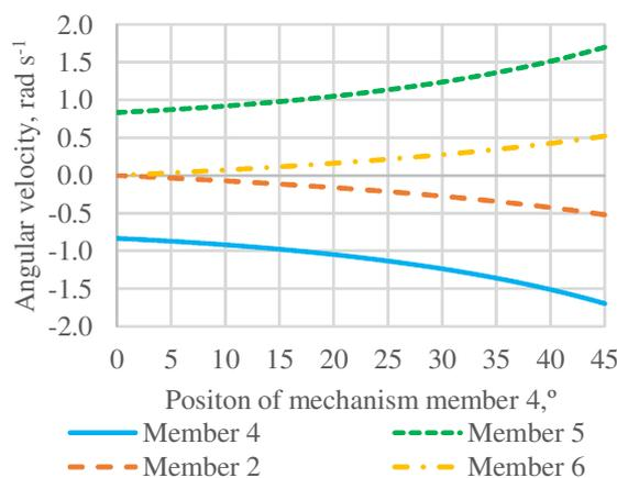
Fig. 6. Angular velocity of rhomboid mechanism links
