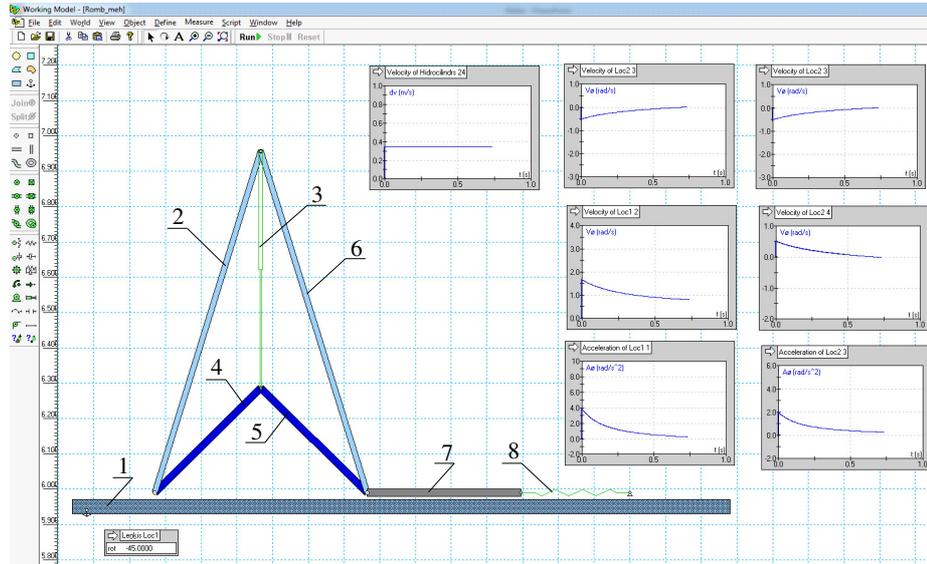
Fig. 3. Rhomboid pressing mechanism in Working Model software: 1 – base; 2, 4, 5, 6 – links of mechanism; 3 – actuator (hydraulic cylinder); 7 – piston; 8 – spring (pressing material characteristics)
