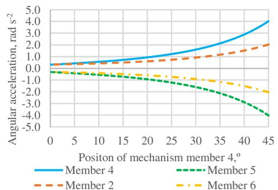
Fig. 7. Angular acceleration of rhomboid mechanism links
