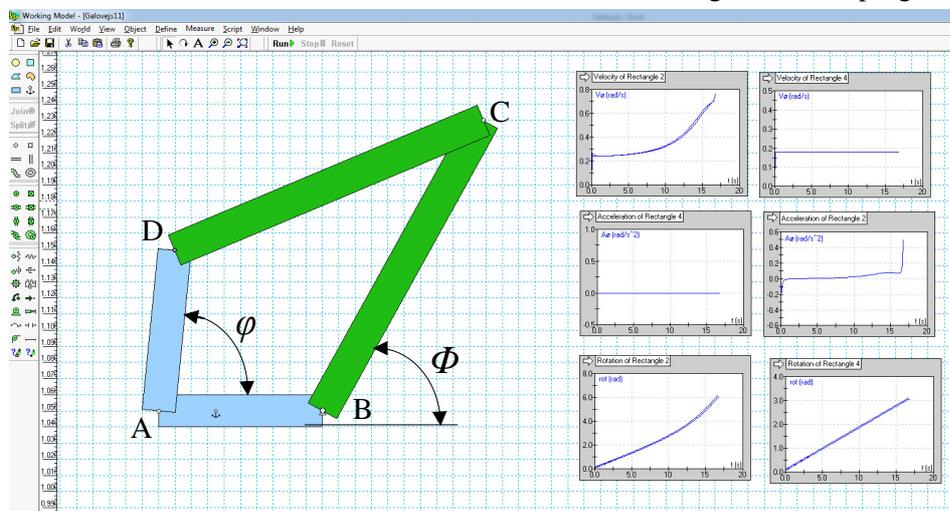
Fig. 2. Galloway mechanism simulation in Working Model software
