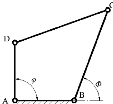
Fig. 1. Rhomboid mechanism with Galloway proportions of links
